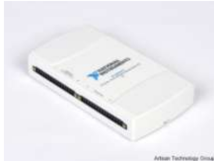
Figure 3. Function generator NI USB-6211 used in XacQuan.
