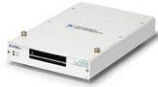
Figure 3. Function generator NI USB-6221 used in XacQuan.
